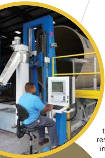
This fully automated cutter not only produces perfectly cut pipes, but since cutting is done in a wet environment, no dust is generated as with past methods.
