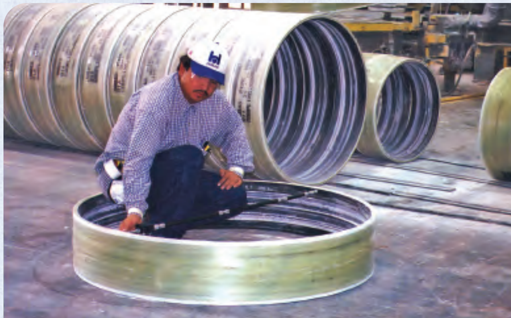
THE MOLDED ID OF THE FWC COUPLING SEALS TO THE MOLD SMOOTH EXTERIOR OF THE HOBAS PIPE FOR A PERFECT SEAL. DIMENSIONS ARE ROUTINELY VERIFIED.
